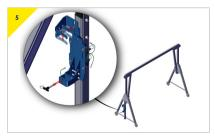
Prepare the bracket to recieve the device and remove the bolt from the bottom connector and loosen the top connector.
