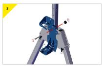
> Insert the supplied M12 top bolt and secure.
