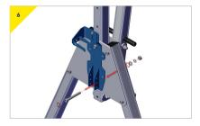
Insert the bottom M16 bolt supplied with bracket and secure.
