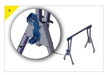
Prepare the bracket to receive the device, make sure all the bolts for the bottom connector have been tightened. Remove the bolt from the bottom connector and loosen the top connector.
