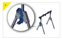
Prepare the bracket to recieve the device, make sure all the bolts for the bottom connector have been tightened. Remove the pin from the bottom connector and loosen the top connector.
