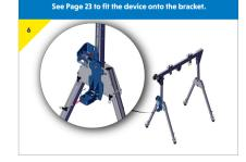
Prepare the bracket to recieve the device, make sure all the bolts for the bottom connector have been tightened. Remove the pin from the bottom connector and loosen the top connector.
