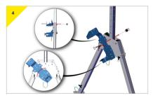
Remove the top bolt whilst holding the bracket on an angle.
