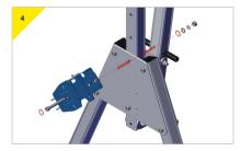
Present the bracket to the trap plate, insert and secure the M16 top bolt supplied with the bracket.
