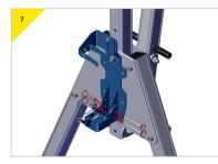
> Re-assemble the bracket to the plate.
