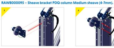
> Present the sheave bracket to the top of the column.
