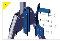
> Re-assemble the bracket to the plate.
