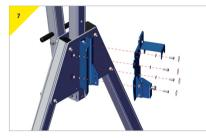
> Re-assemble the bracket to the plate.
