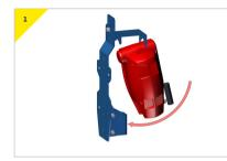
> Present the device onto the bracket.
