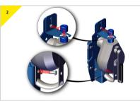
Insert the bottom bolt to secure the device into position. Adjust the top connector in the suitable position and secure by tightening the bolt.
