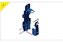
> Before attaching the bracket to the device, dissemble the bracket.
