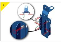
> Adjust the width of the wings to 2 1/2" (63.5mm) and fit the bracket onto the Porta Davit Quantum backstay.
