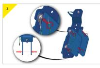
Adjust the width of the wings to 2 1/2" (76.2mm) and fit the bracket onto the Porta Davit Quantum backstay.
