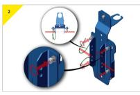
> Adjust the width of the wings to 3" (76.2mm) to fit on the winch column.
