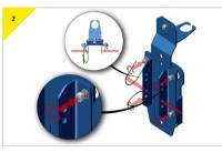
> Adjust the width of the wings to 3" (76.2mm) to fit on the T davit column section.
