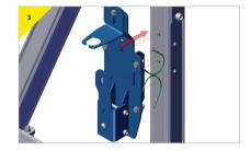
> Present the bracket onto the winch column.
