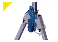
> Re-assemble the bracket to the plate.
