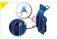
Adjust the width of the wings to 2" (50.8mm) to fit on the Porta Davit 500 backstay.
