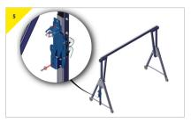
Prepare the bracket to recieve the device. Remove the bolt from the bottom connector and loosen the top connector.
