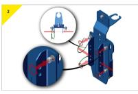
> Adjust the width of the wings to 3" (76.2mm) and fit the bracket onto the Porta Davit Quantum column.
