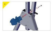
> Present the bracket to the trap plate, insert and secure the M16 bolt supplied with the bracket.
