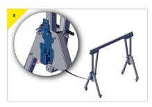
Prepare the bracket to receive the device, and remove the bolt from the bottom connector and loosen the top connector.
