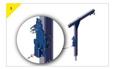
Prepare the bracket to recieve the device. Remove the bolt from the bottom connector and loosen the top connector.
