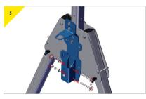
> Re-assemble the bracket to the plate.
