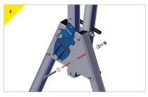
Remove the bottom bolt from the trap plate, and wing the bracket into position.
