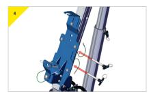
Insert the pins provided with the bracket.
