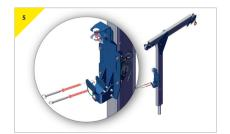
Prepare the bracket to recieve the device. Remove the pins from the bottom connector and loosen the top connector.
