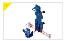
Defore attaching the bracket to the device, dissemble the bracket. The bottom connector needs to be removed before attaching to the Porta gantry Rapide.
