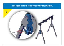
Prepare the bracket to recieve the device, make sure all bolts for the bottom connector have been tightened. Remove the pins from the bottom connector and loosen the top connector.
