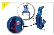
Adjust the width of the wings to 3" (76.2mm) and fit the bracket onto the Porta Davit Quantum column.
