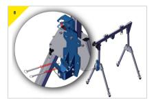
Prepare the bracket to receive the device, make sure all bolts for the bottom connector have been tightened. Remove the pins from the bottom connector and loosen the top connector.
