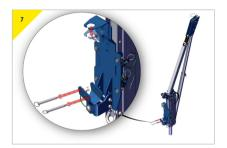
Prepare the bracket to receive the device and remove the bolt from the bottom connector and loosen the top connector.
