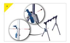
Remove the top bolt whilst holding the bracket on an angle..
