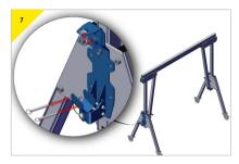
Reassemble the bracket. Make sure all the bolts for the bottom connector have been tightened. Prepare the bracket to receive the device, remove the pins from the bottom connector and loosen the top connector.
