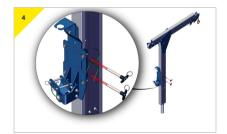
Insert the pins provided with the bracket.
