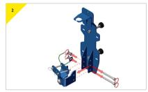
Before attaching the bracket to the device, dissemble the bracket. The bottom connector needs to be removed before attaching to the Porta Gantry Rapide.
