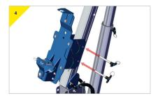
Insert the pins provided with the bracket.
