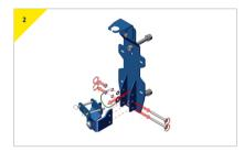
Disassemble the bracket. The bottom connector needs to be removed before attaching to the Porta Gantry.
