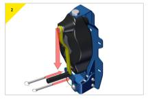
Place the device into the bottom connector and insert the bottom pins to secure the device into position. Make sure the pins are fully secure and engaged.
