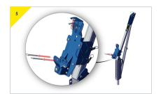
Prepare the bracket to receive device, remove the pins from the bottom connector and loosen the top connector.
