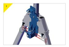
Reassemble the bracket. Make sure all the bolts for the bottom connector have been tightened.
