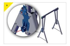
Prepare the bracket to receive the device, and remove the bolt from the bottom connector and loosen the top connector.
