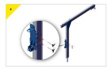
Insert the pins provided with the bracket.
