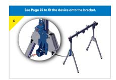
Prepare the bracket to recieve the device and remove the bolt from the bottom connector and loosen the top connector.
