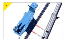
Insert the pins provided with the bracket.
