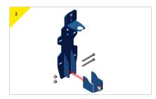
> Remove the bottom connector from the bracket before commencing the assembly.
