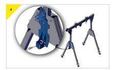
Prepare the bracket to recieve the device and remove the bolt from the bottom connector and loosen the top connector.
