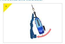
> Present the device onto the bracket.
