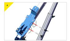
Insert the pins provided with the bracket.
