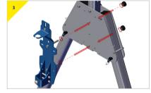
Present the bracket to the trap plate, insert and secure the top and bottom M12 bolts supplied with the bracket.
