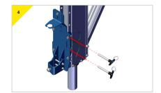
Insert the pins provided with the bracket.
