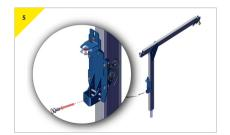
Prepare the bracket to recieve the device. Remove the bolt from the bottom connector and loosen the top connector.
