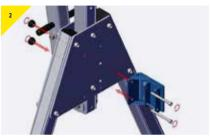
Present the bracket to the trap plate, securing using the M12 bolts supplied.
