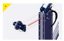
> Present the sheave bracket\* to the upper-most holes of the column.
