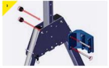
> Present the bracket to the trap plate, securing using the M12 bolts supplied.
