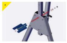
Present the bracket to the trap plate, securing using the M16 bolt provided.
