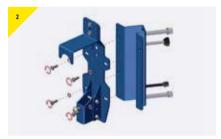
**)** Disassemble the bracket, separating the back plate from the faceplate.
