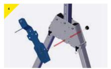
> Present the bracket to the trap plate and secure using the M12 bolt provided.
