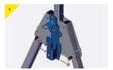
> Reassemble the bracket using all bolts.
