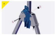
Straighten the bracket and secure using the top bolt.
