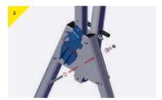
> Remove the bottom bolt from the trap plate.
