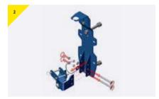
Disassemble the bracket.
