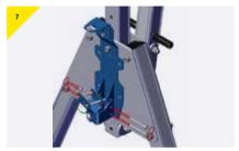
> Reassemble the bracket using all bolts.
