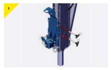
> Present the bracket to the column and secure using the pins provided.
