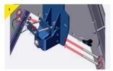
> Reassemble the bracket using all bolts.
