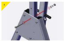
> Remove top bolt from trap plate.
