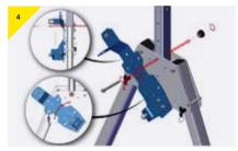
> With the bottom bolt in place, rotate the bracket in order to remove the top bolt.
