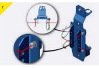
> Adjust the width of the wings to 63.5mm to fit comfortably on the backstay.
