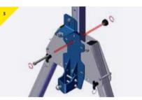
> Straighten the bracket and secure using the top bolt.
