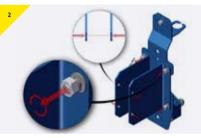
> Adjust the width of the wings to 63.5mm to fit comfortably on the backstay.
