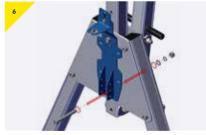
Carefully align the backplate and secure into the bottom hole on the trap plate using the M16 bolt provided.
