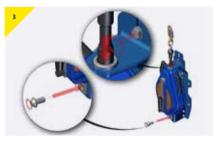
Secure the Device by reinserting the bottom bolt. Tighten the top connector into a secure position.
