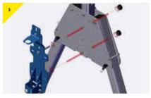
> Present the bracket to the trap plate and secure using the M12 bolts provided.
