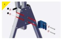
Present the bracket to the trap plate using the centre holes, securing with the M12 bolts.
