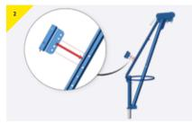
> Remove the pins and present the bracket to the backstay, aligned to the holes as shown.
