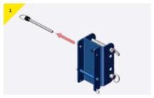
> Remove the pin from the bracket.
