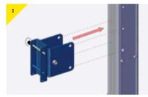
> Remove the pins and present the bracket to the column, aligned to the holes as shown.
