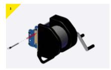
Adjust the position, placing the device attachment arm into the bracket as shown and secure with the pin.
