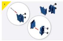
Disassemble the bracket by removing the pins, bolts and separating the pieces.
