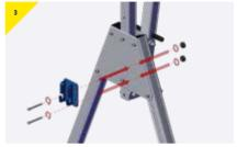
Present the bracket to the trap plate as shown, secure both M12 bolts through the correct holes as shown.
