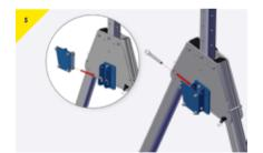
Reassemble the bracket using the pins provided as shown. First the lower pin and slide into place and secure with the top pin.
