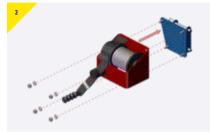
Present the device to the bracket, resecure the bolts using the washers and nyloc nuts.
