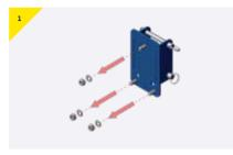
Remove the washers and nyloc nuts from the bracket.
