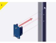
> Remove the pins and present the bracket to the winch column, aligned to the holes as shown.
