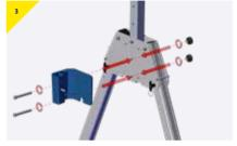
> Present the bracket to the trap plate and secure in the central holes using the M12 bolts supplied.
