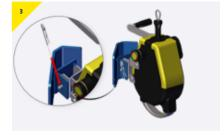
> Secure the pin in position using the R-Clip provided.
