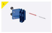
> Remove the pin from the bracket.
