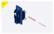
> Remove the pin from the bracket.
