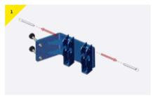
> Remove the pin from the bracket.
